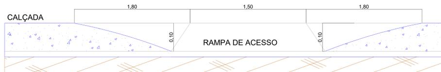
**DETALHE MEIO FIO E RAMPA SEM ESCALA**
